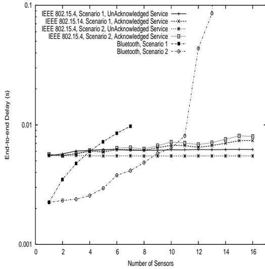
Fig. 3. Delay as a function of number of sensors
