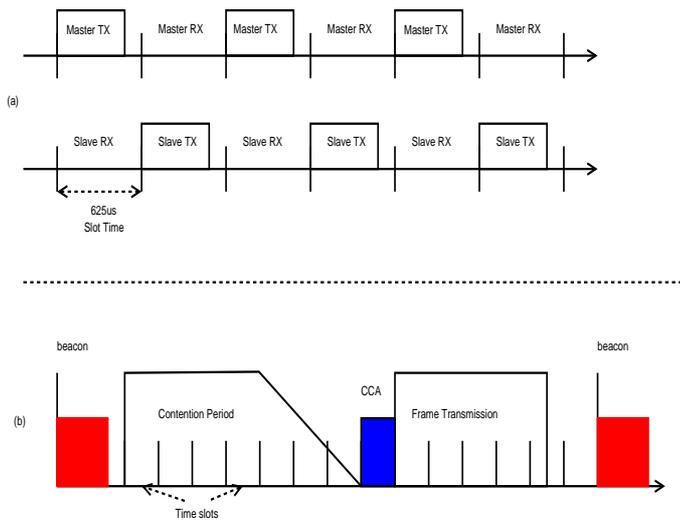
Fig. 1. WPAN structure: (a)Bluetooth (b)Slotted 802.15.4
