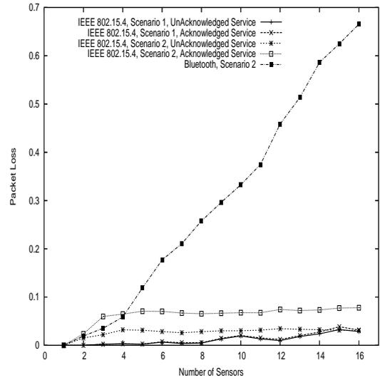
Fig. 4. Packet Loss as a function of number of sensors
