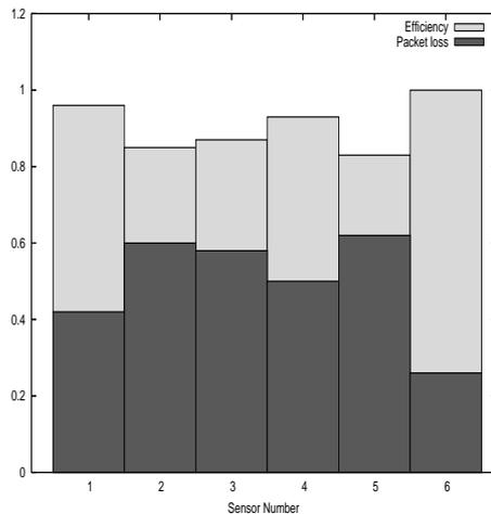
Fig. 7. Packet Loss and Efficiency per IEEE 802.15.4 Sensor
