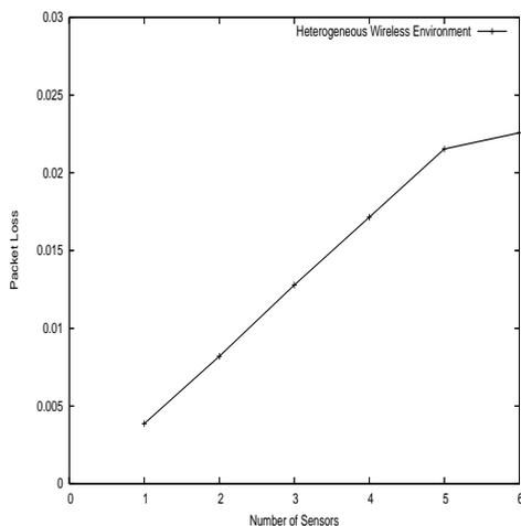
Fig. 8. Bluetooth Packet Loss as a function of the number of IEEE 802.15.4 sensors
